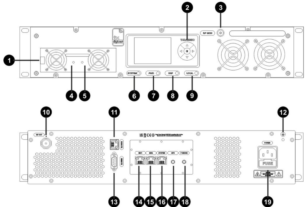
1. **PSU RETAINING CLIP** Push to the right in order to release the PSU, then pull forward gently, using the handle.
